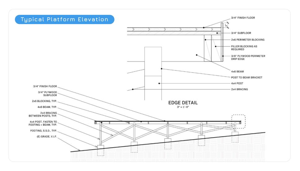
Measure, mark and lay out concrete blocks or pour footings according to plans and level.
